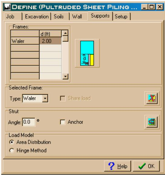
In this case a wale with tiebacks 2' from the top of the wall is added. As a result, the bending moment falls to within the allowable bending moment of the pultruded sheet piling. It is important to carefully note the wale support load per unit length of wall, as this is essential in proper tieback design for any wall design.
